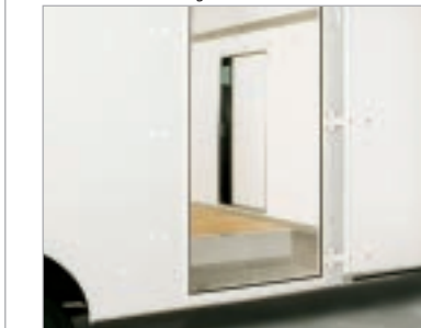
Step-Saver side swing door with low step well for easy curb access and low-height cab-access door
