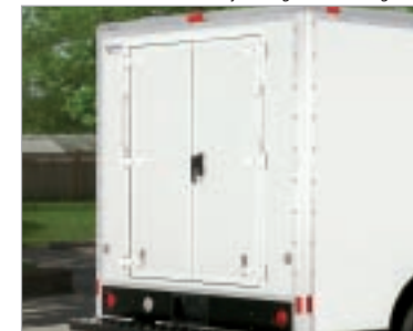
48 1/2" rear double doors for easy loading and unloading
