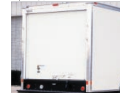
Full-width, roll-up rear door with side seals for easy access in tight delivery spaces
